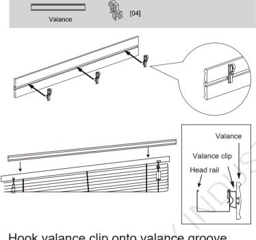
Hook valance clip onto valance groove first then hook onto head rail as above picture shows.
